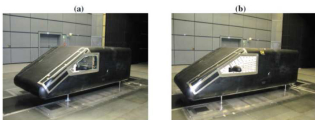
Figure 39. Wind-tunnel test: (a) glass module, (b) sensor module
