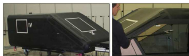
Figure 29. Noise Reduction (NR) measurements performed on several patches around the SAE body.
